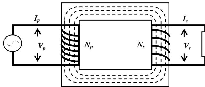
Fig. 1 Schematic transformer structure
