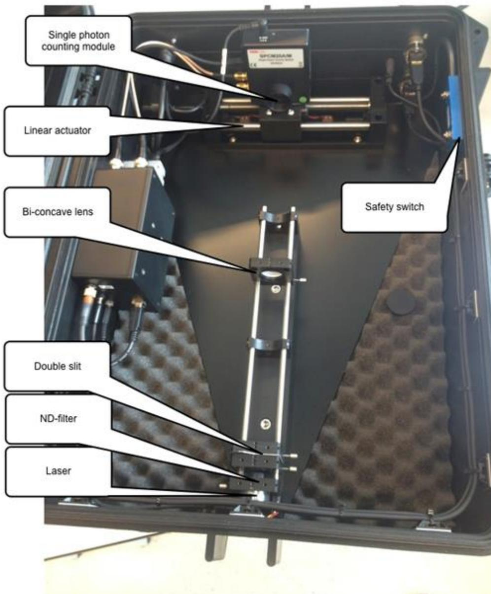
Figure 1 Single Photon interference set-up in suitcase
