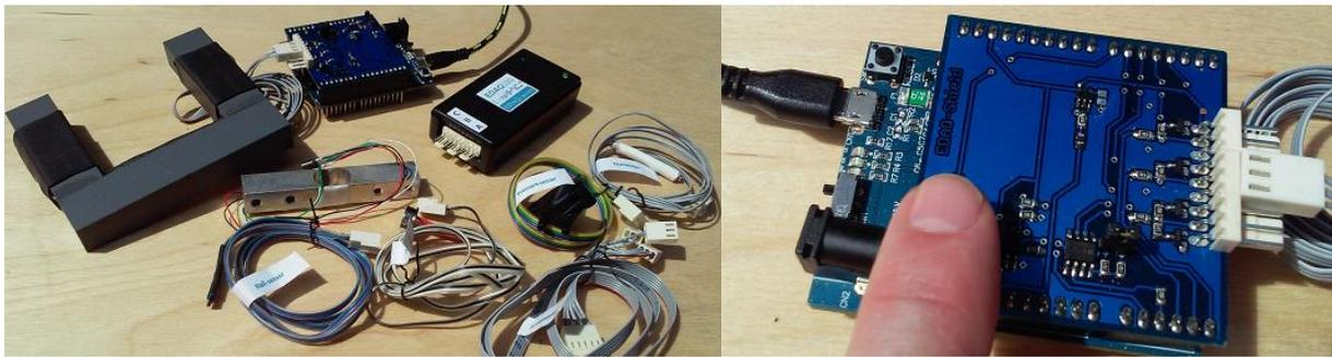
Fig. 2 On the left: EDAQ530 and EDAQuino with various sensors. On the right: EDAQuino measures blood flow in a fingertip.
