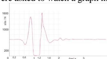
Fig. 1 A force (time) graph presented to students during the test. A squat jump on a force plate [5].
