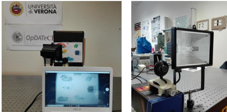
Infrared reflectography experiment with a web camera on a painting mock-up .
