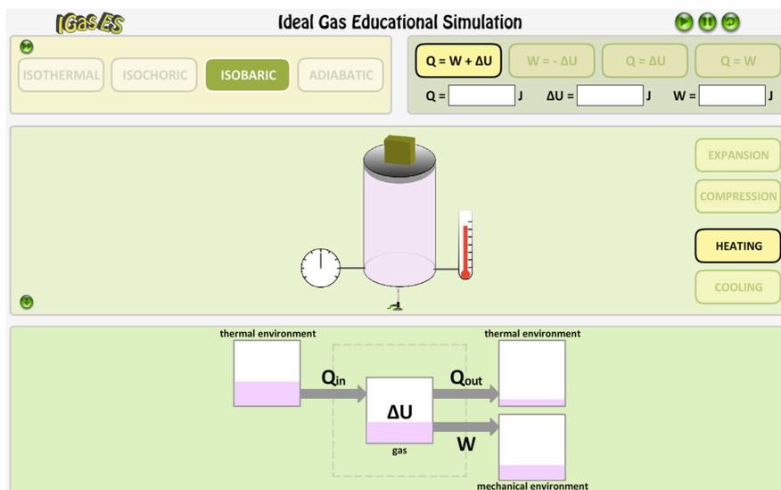
Fig. 1 Snapshot of IGasES: isobaric heating at equilibrium state
