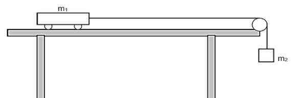
Fig. 1 Two masses connected by a massless string
