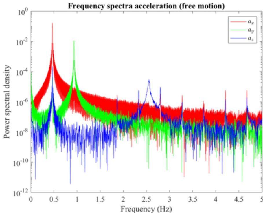
Fig. 1 Lomb-Scargle transform of 3-axis accelerometer data from a mobile phone attached to a knife-edge physical pendulum. The z-axis is normal to the plane of the motion and the y-axis along the radial direction. [Image by Duncan Carlsmith]
