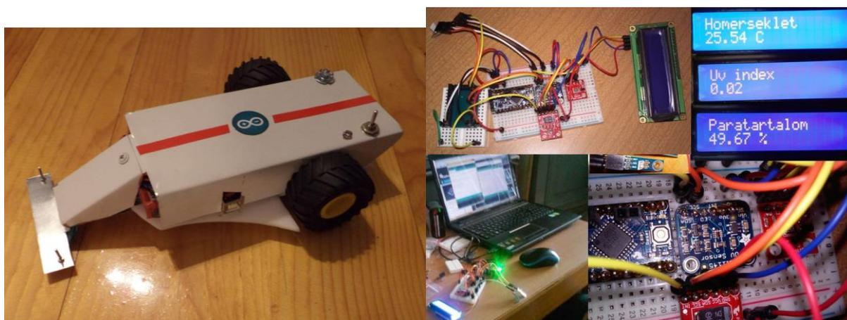
Fig.3. Arduino controlled line follower and mini meteorological station
