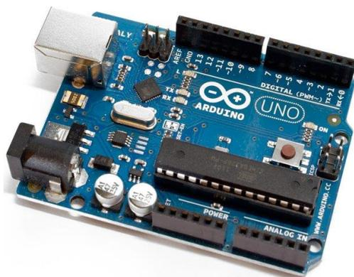
Fig. 1 The Arduino Uno board
