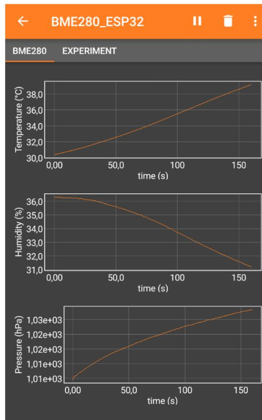
Fig. 1 Measurement of the pressure, temperature and humidity as a function of time inside of a glass jar, which was placed inside a pot of boiling water.
