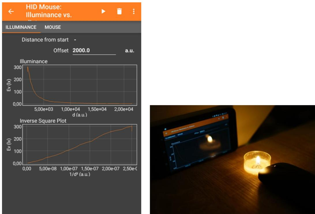
Fig. 1: Illuminance of a candle at different distances to measure the quadratic correlation.
